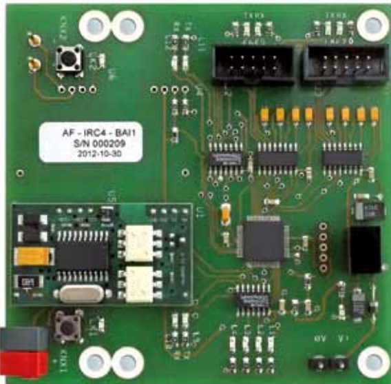
Fig. 4. The interface board connected between a KNX bus and the security system control panel
