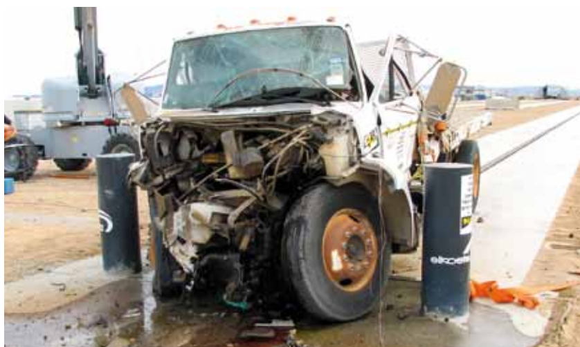
Fig. 6. Anti-ram bollards tests – the truck after crush test Photo – Gunnebo Polska
