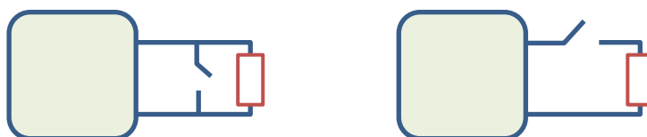
Figure 1. Left: normally open Sensor (parallel resistor). Right: Normally Closed Sensor (serial resistor).
