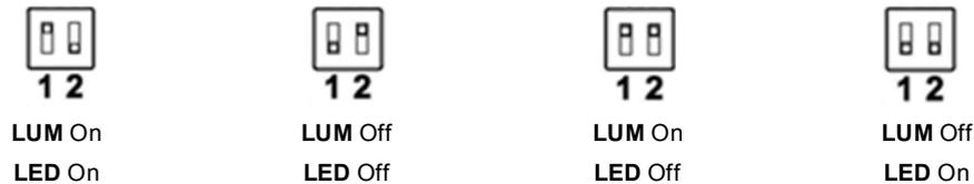
Figure 4. Positions of the Double Micro-Switch
