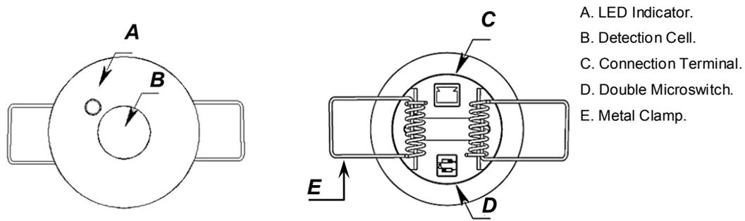
Figure 2. Element Diagram (models ZN1IO-DETEC and ZN1IO-DETEC-N)
