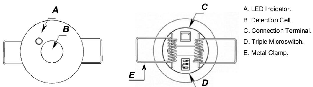
Figure 3. Element Diagram (models ZN1IO-DETEC-P and ZN1IO-DETEC-X)
