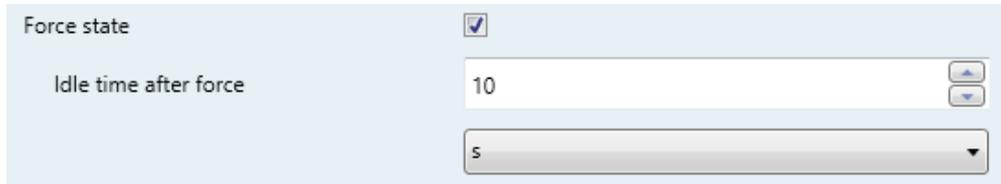
The screenshot shows a configuration panel for 'Force state'. At the top, there is a checkbox labeled 'Force state' which is checked. Below it, there is a label 'Idle time after force' followed by a numeric input field containing the value '10'. To the right of this field are up and down arrow buttons. Below the input field is a dropdown menu with a downward-pointing arrow, currently displaying the value '5'.
