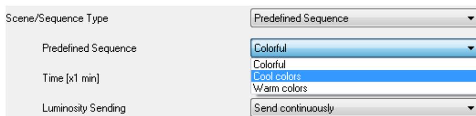
These sequences have 5 steps (or smooth transitions between different colors) of determined duration. They are **cyclical**, so when the last step of the sequence finishes, it will start again from the beginning (first step) automatically. The default duration of every cycle is 1 minute, but it can be modified in the box **Time** (t), writing a value in the range [1...255], in minutes.
