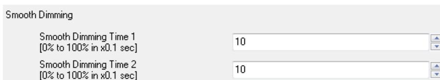
Smooth Dimming Time 1 and 2 may be modified in execution time, via the communication objects "Dimming Speed 1" and "Dimming Speed 2", respectively. Please see the Table 3.1 to know the relation between several dimming speed values (the most common ones) and its associated dimming times.
