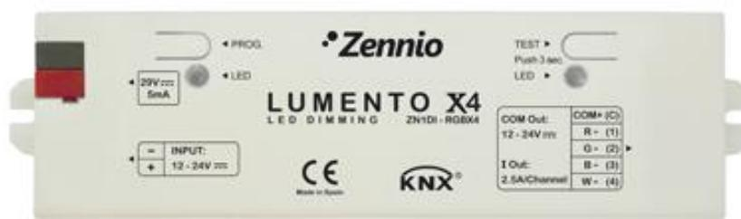
Figure 1.1. Lumento X4 LED controller
